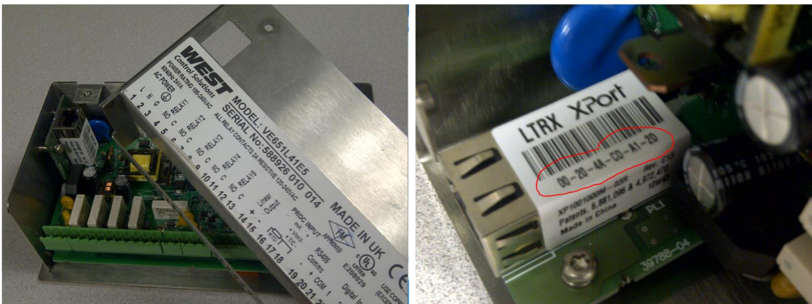
Figure 8-3 Protocol 3 remove cover and record MAC address
